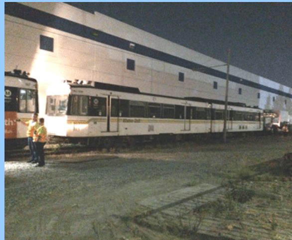
Car 129 has now been placed at the end of the siding next to the building. Later that day, the truck behind it will push Car 129 across Washington Boulevard on a track with no overhead wire to a short section of track adjacent to the Wilmington Station. The car will be loaded onto the trailer as shown in our previous issues while passengers on the northbound Blue Line trains pass by totally oblivious to what is going on.
